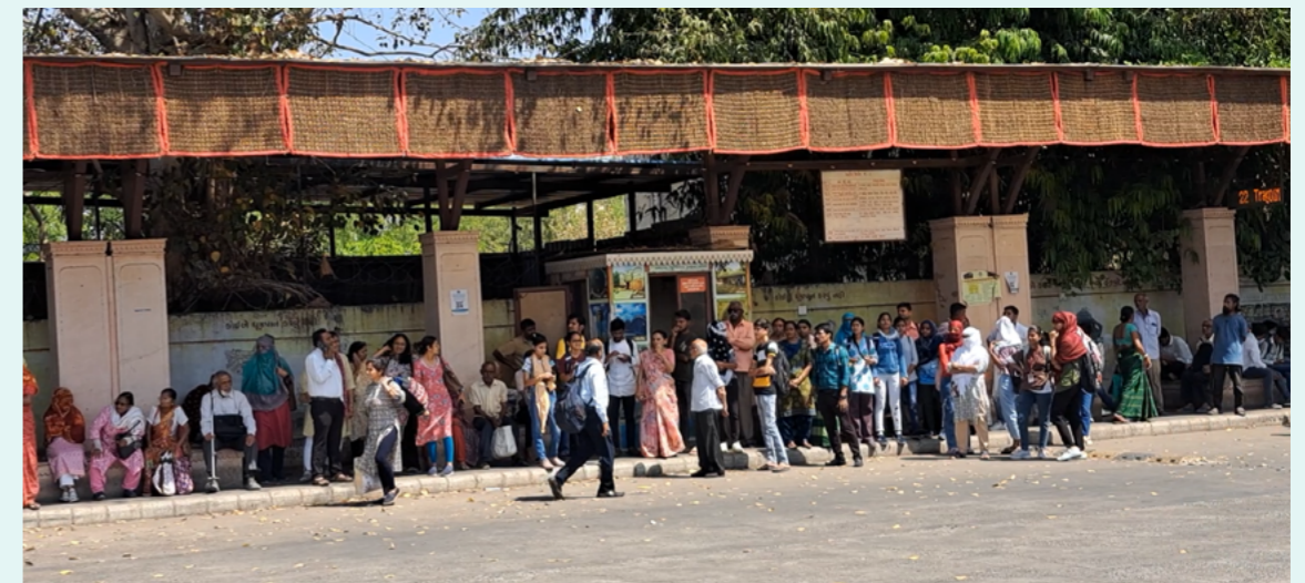
Bus stop in Ahmedabad, India with high-pressure misting systems drop ambient temperatures by 6-7°C and traditional vetiver grass and straw curtains naturally regulate heat and provide shade. Source: Mahila Housing Trust.
