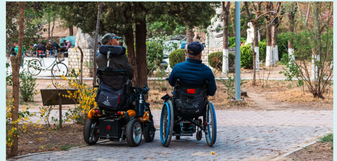
Permeable and even-surfaced pavements reduce storm water runoff and allow people in wheelchairs to comfortably access all parts of the park
