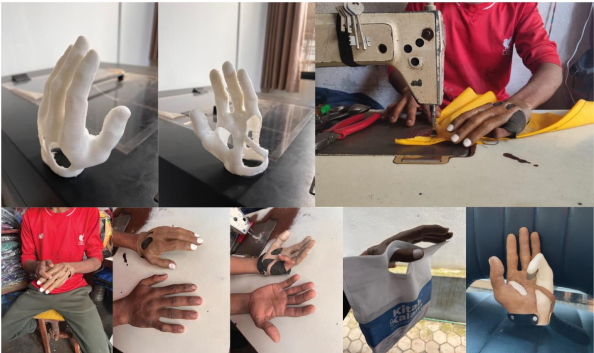
Figure 20: Printing and user testing on v1
