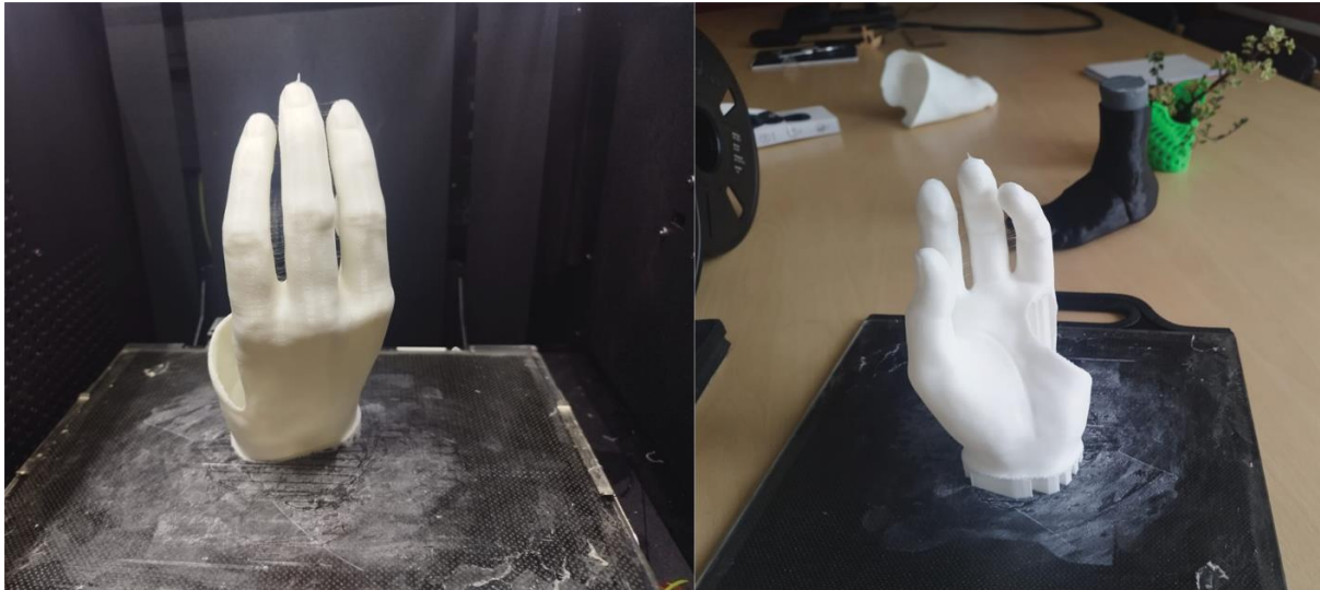
Figure 23. Printing of v3 in TPU flexible filament
