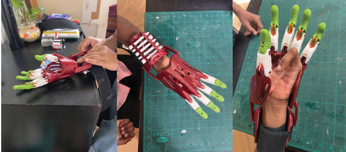
Figure 15: An adapted design for an actuating prosthesis based on an open source design 49
