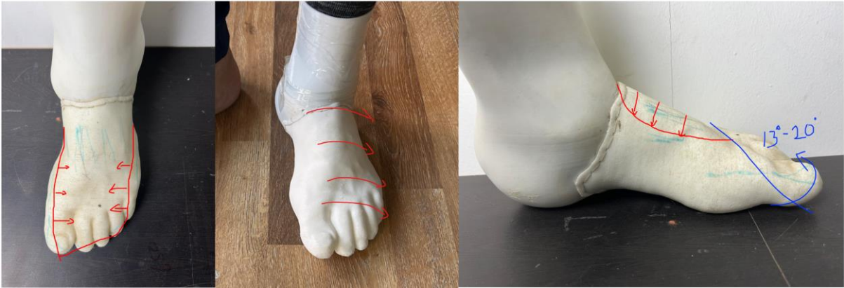
Figure 10 a) Size Reduction Marks; b) Natural Tendency to Incline towards outer left side ; c) Volume reduction and steep slope (red), Toe break angle and position mark (blue)
